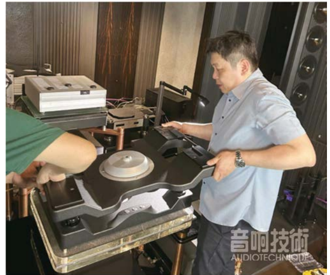
Edward is assembling the middle layer with captured bearing
