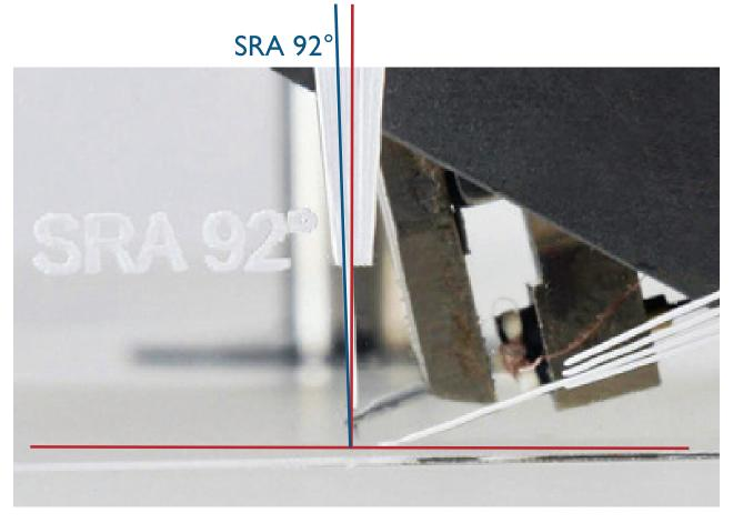
If you align your stylus to 92°, you will find this a position which will give you a very close to optimum angle of your contact area with most (but not all) modern cartridges and most modern cut records.
